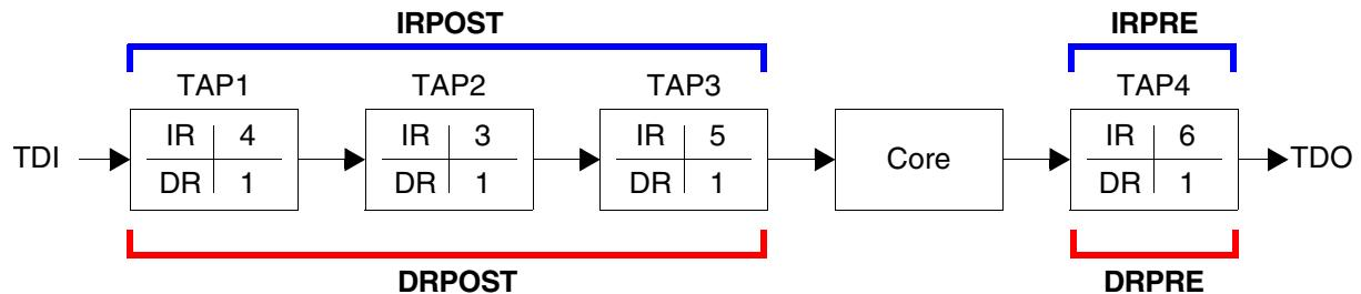
**IR:** Instruction register length    **DR:** Data register length    **Core:** The core you want to debug
