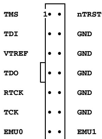
This is a standard 14 pin double row (two rows of seven pins) connector (pin-to-pin spacing: 0.100 in.).
