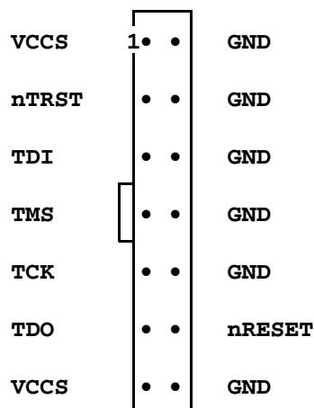
This is a standard 14 pin double row (two rows of seven pins) connector (pin-to-pin spacing: 0.100 in.).
