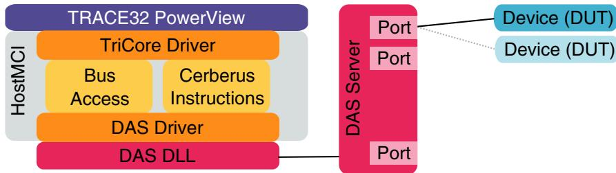
TRACE32 runs completely on a host computer. This includes the debugger back-end (HostMCI) containing the high-performance multicore debug driver; the same driver that is also used together with real Lauterbach hardware.
