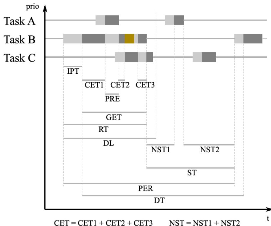
Depending on the recorded events and the available trace data, TRACE32 is able to evaluate these events, too. Some of the **Trace.STATistic** commands allow the display of these parameters (by using the **/ARTI** option) or directly accept the AUTOSAR timing parameter as item. See the next chapter for details.
