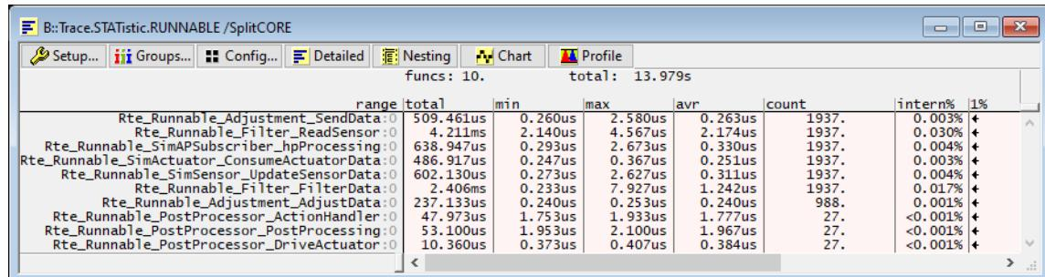
The screenshot shows a software interface titled 'B::Trace.STATistic.RUNNABLE /SplitCORE'. The window contains a table with the following columns: range, total, min, max, avr, count, intern%, and 1%. The table lists various RTE runnable functions with their respective timing statistics. For example, 'Rte\_Runnable\_Adjustment\_SendData:0' has a total time of 509.461us, while 'Rte\_Runnable\_PostProcessor\_Start:0' has a total time of 13.979s.
