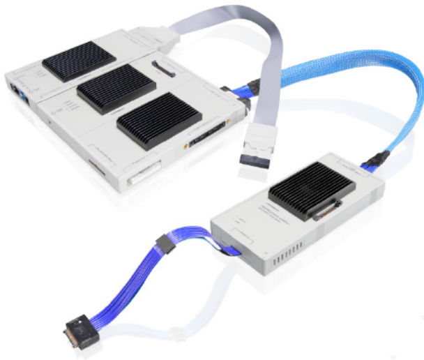
Picture: Aurora 2 Preprocessor connected to a PowerTrace Serial, IDC20A Debug Cable connected to PowerDebug module.
