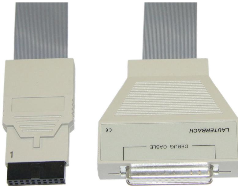
Beginning with September 2008, the bidirectional debug cables completely replaced the unidirectional OCDS debug cables. In JTAG mode they are backwards compatible.
