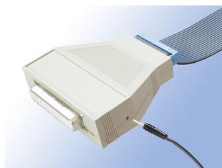
There is a single cable contact on the casing of the debug cable which can be used to detect if the JTAG connector of the debugger is tristated e.g. when **SYStem.Mode NoDebug** is active. If so, also this signal is tristated, otherwise it is pulled low. This can be used, e.g. for triggering a Logic Analyzer. See the **SYStem.LOCK** command for additional information.
