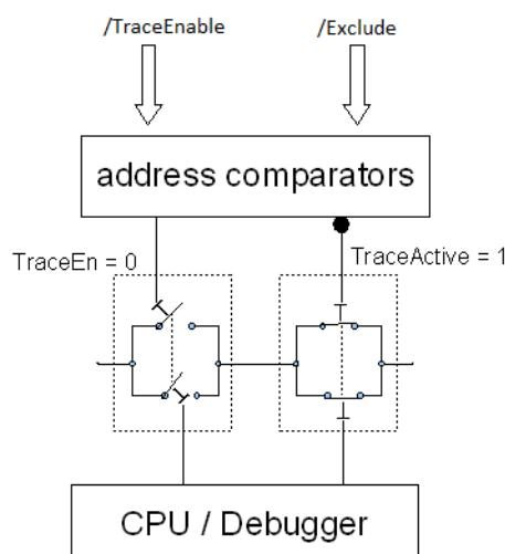
Two register bits control the generation of trace data: *TraceEnable* and *TraceActive*. Both must be set to '1' in order to enable the trace (AND operation). They can either be accessed by the IP address comparators or by the CPU / debugger.
