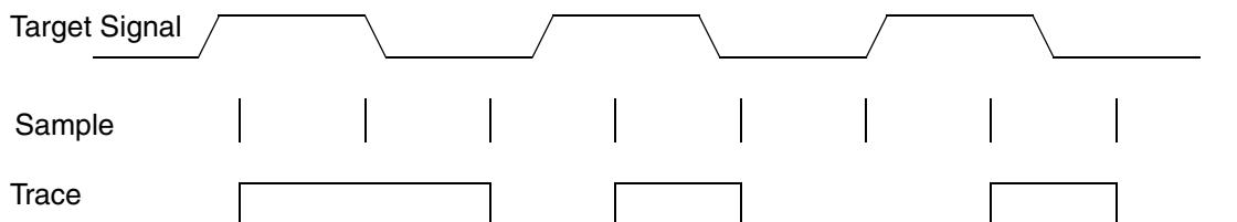
State Recording is the appropriate method to trace synchronous bus protocols. A typical application is a clocked SDRAM bus where valid data is driven on the bus relative to the SDRAM clock.
