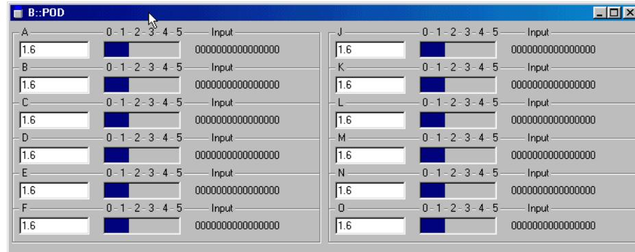
The POD window shows the selected threshold levels and the activity of the target signals.
