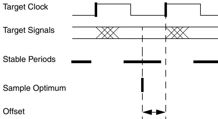
To find Stable Periods the PowerIntegrator includes a comfortable analysis option called '**TestFocus**'. It does a signal analysis in the range of -3ns to +6ns around the clock edge. The signal has to be 'quiet' for a quarter of the target clock period to be marked as stable period.
