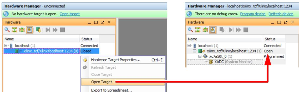
3. Connect to the target by right-clicking this sub-entry, and then select **Open Target** from the popup menu. Its status should change to “Open”, and show sub-entries for the JTAG components.
