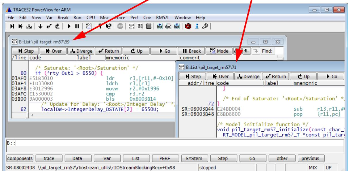
You can navigate from the source code displayed in a **List** window of TRACE32 PowerView back to the corresponding Simulink block.
