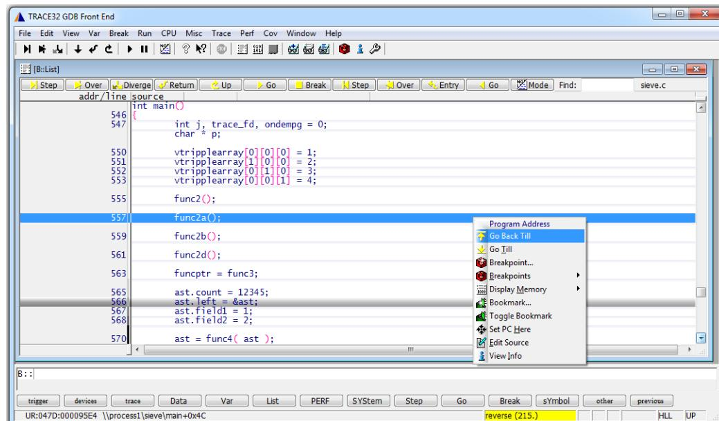
The TRACE32 GDB Front-End supports debugging the Linux kernel using KGDB. Please note that it is only possible to debug the kernel space. Debugging the user-space as supported by the TRACE32 Stop Mode Debugging for Linux is not possible.
