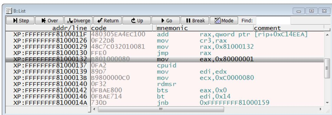
From now on, the Linux kernel runs completely in logical address space. The symbols are all bound to these logical addresses, so simply load the Linux symbols without any offset:
