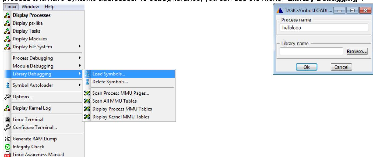
This menu point is based on the TRACE32 command **TASK.sYmbol.LOADLib**.
