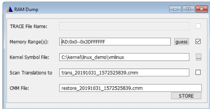
After pushing the STORE button, the dialog will save the RAM contents as well as important register values and will generate a `restore_<...>.cmm` script that can be used to restore the system state on the TRACE32 instruction set simulator.
