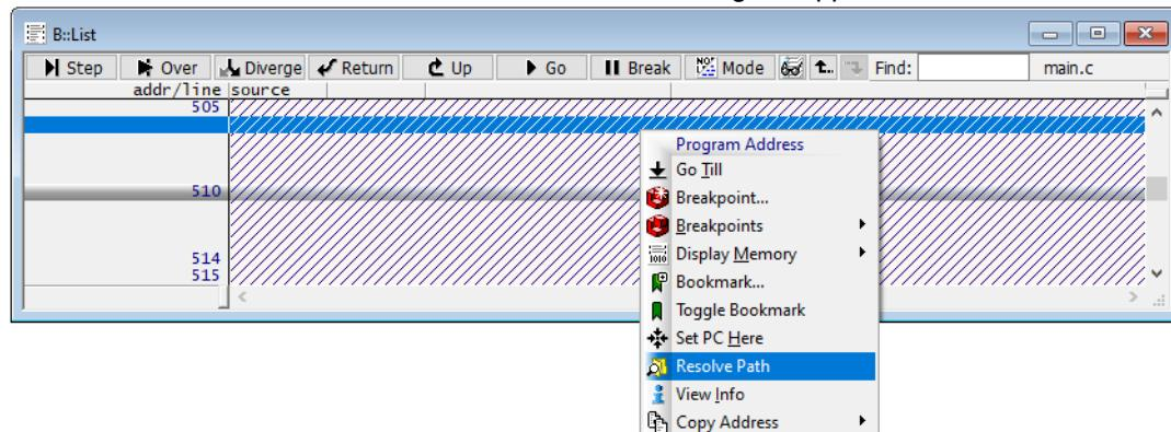
You just need then to browse to the source code file. The result of **Resolve Path** is a source path translation which will be used to locate all kernel source code files. This means that you have to resolve the path of a single source code file and all other kernel sources will be automatically found by TRACE32.
