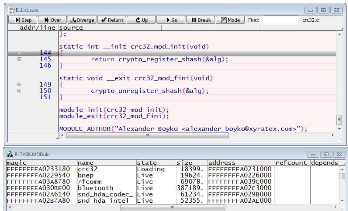
If the Symbol Autoloader cannot find the module's ko file, a file browser will pop-up. If you want the debugger to automatically find your kernel module, you need to add its path to the TRACE32 search paths using the command **sYmbol.SourcePATH.SetDir**. Alternatively, you can define a ROOTPATH using the command **TASK.sYmbol.Option ROOTPATH**. Please refer to "["OS Awareness Manual Linux"](#)" (rtos\_linux\_stop.pdf) for more information about this command.
