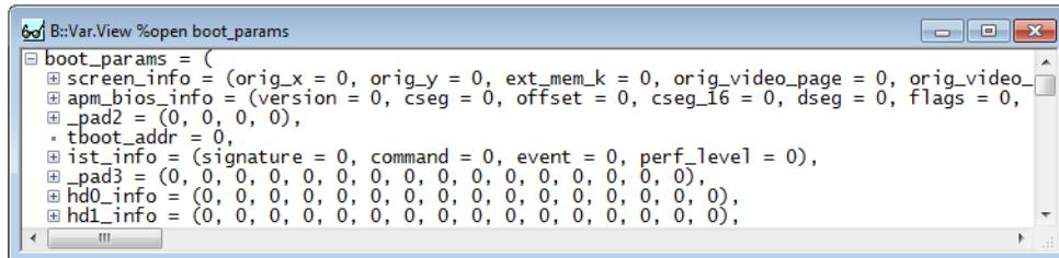
In the following example, we first set the `boot_params` area to zero and then set the parameters `alt_mem_k`, `hrd.type_pf_loader`, `hdr.ramdisk_image` and `hdr.ramdisk_size` (since we use a ramdisk as a file system) as well as the boot command line ptr `hdr.cmd_line_ptr`. The offsets of the structure elements are hard coded.
