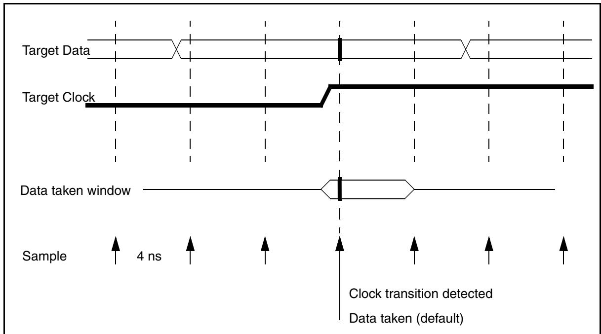
A Target Clock edge is detected by comparing the current sampling against the sampling before. If there is a difference then a clock transition had occurred.
