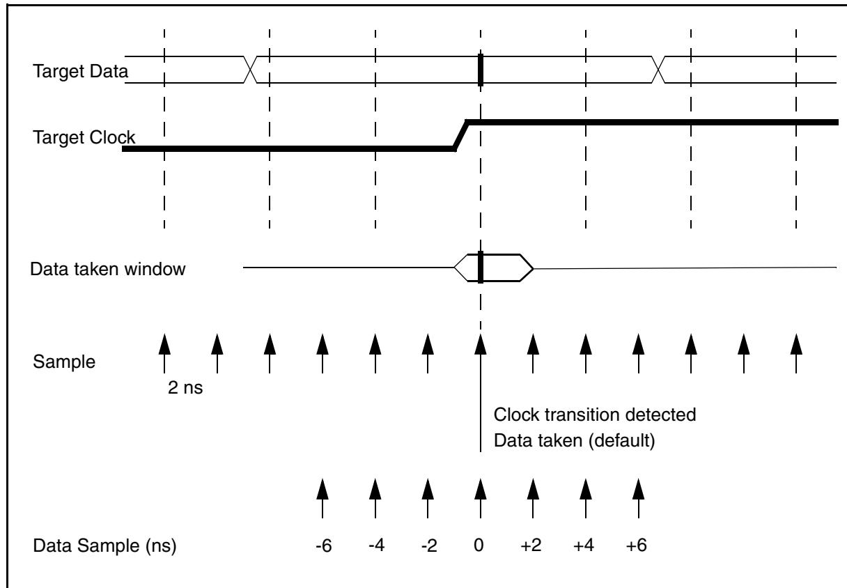
A Target Clock edge is detected by comparing the current sampling against the sampling before. If there is a difference then a clock transition had occurred.
