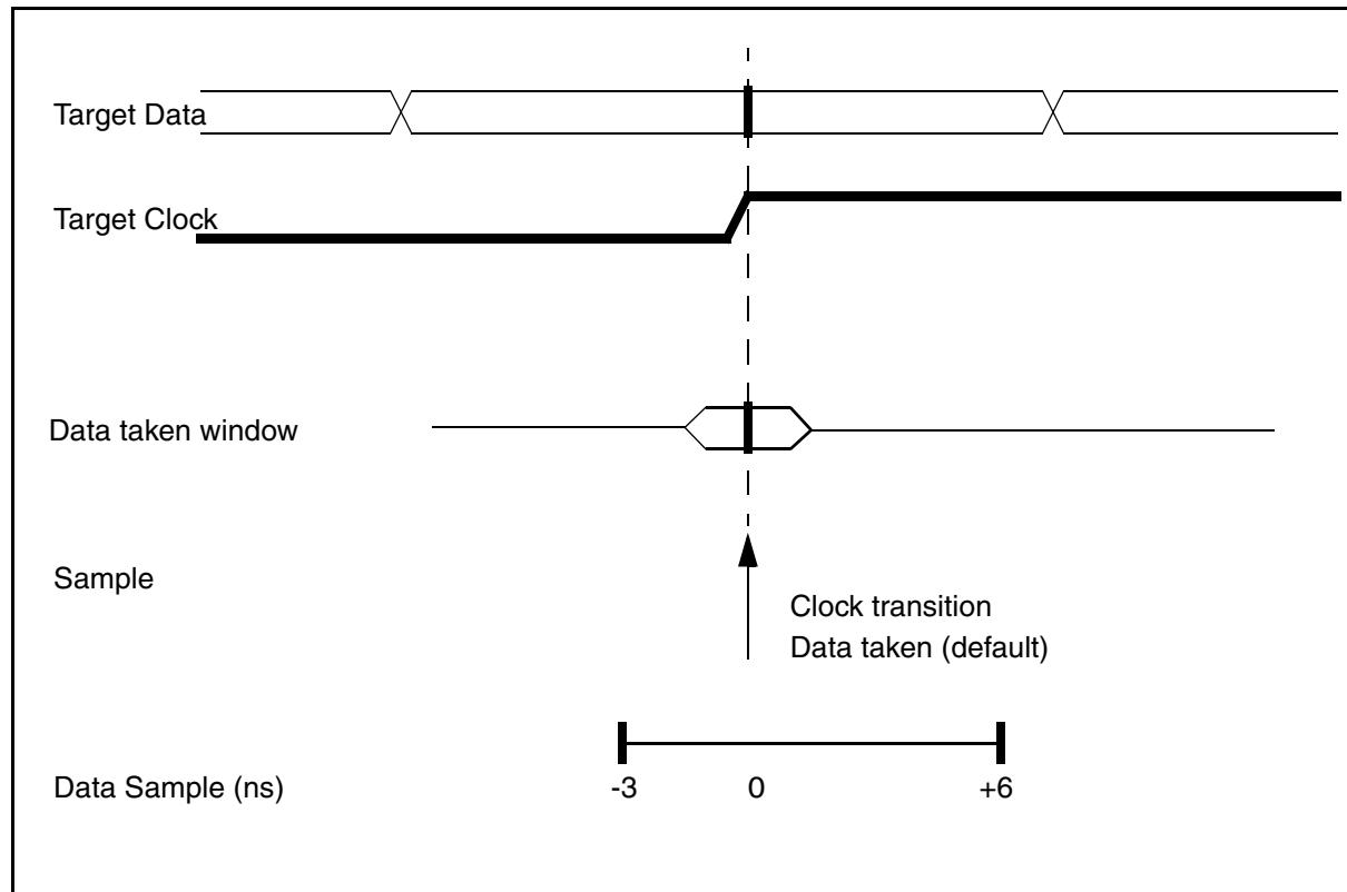
The target clock itself defines the sampling point of the data channels. Data has to be stable for only 1 ns.
