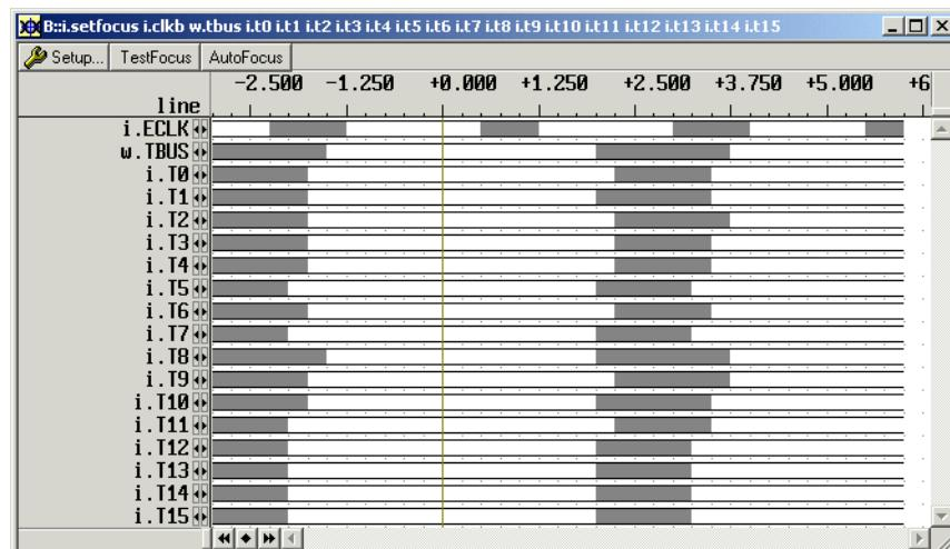
The screenshot shows the measurement for a 200 MHz single data rate bus.
