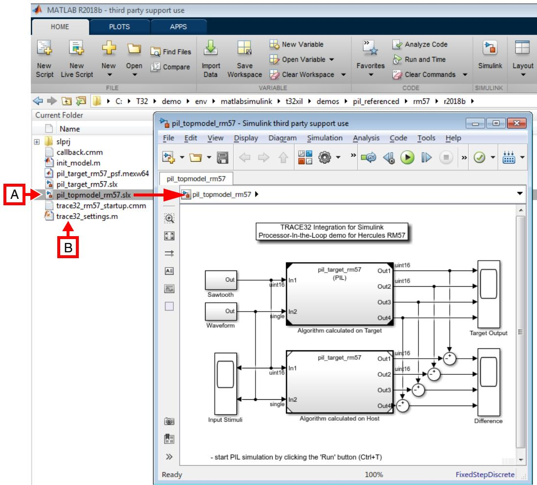
6. Open the file `trace32_settings.m` [B] and increase the communication timeout value of `cfg.Timeout_Transfer`.
