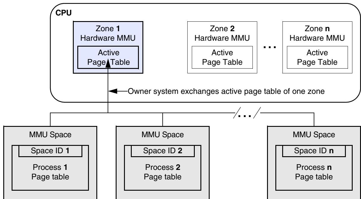
Standard use cases for MMU spaces are operating systems, such as Linux, where processes run on identical virtual addresses and the kernel configures an individual page table for each process. Often, the number of valid MMU spaces is dynamic: during runtime new MMU spaces may be created or removed by the controlling software - for example if an OS creates or terminates processes.
