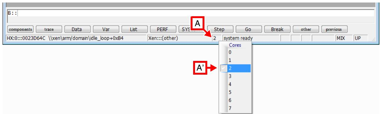
Double-clicking the **Cores** field [A] opens the **CORE.List** window:
