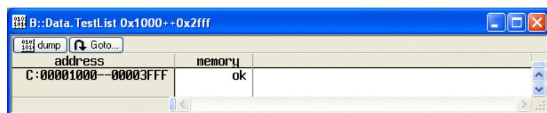
If the result is **read fail** or **write fail**, please check the bus configuration registers for the RAM and the RAM initialization.
