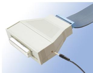
There is a single cable contact on the casing of the debug cable which can be used to detect if the JTAG connector of the debugger is tristated. If tristated also this signal is tristated, otherwise it is pulled low.
