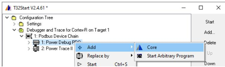
Because two devices are used for debugging, both of them have to be included in the **Podbus Device Chain**.
