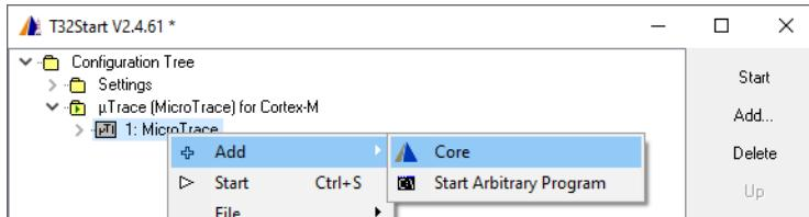
Open the **Core** branch to specify the target core.
