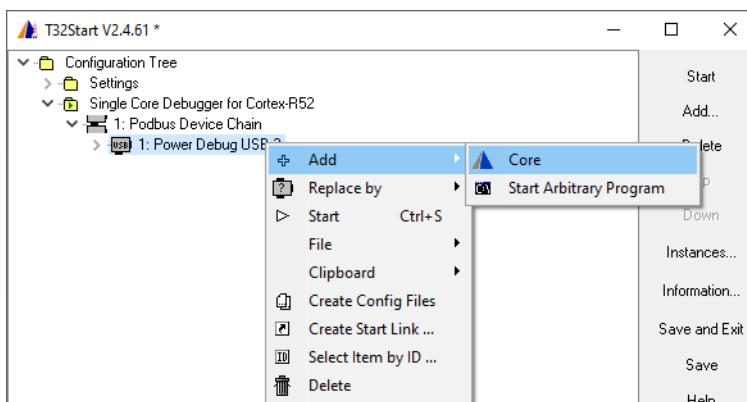
6. Open the **Core** branch to specify Arm as architecture for debugging.
