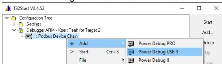
5. Assign the first Core to the **Power Debug USB3**.
