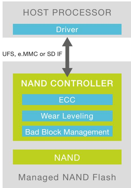
The specific architecture of a managed-NAND device can be extremely sensitive to certain read and write access sequences performed by the host processor under the direction of the application software, especially if these are frequently iterated.
