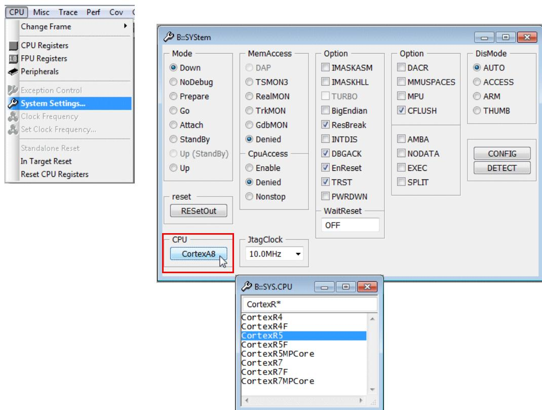
Inform the debugger about the core/chip on your target, if an automatic detection of the core/chip is not possible. Wild card symbols \* or ? are allowed.
