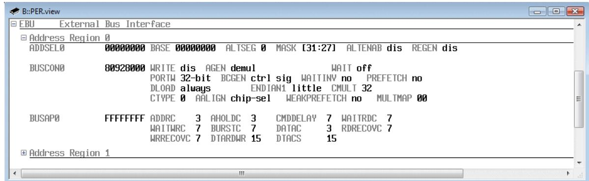
In order to have write access to the used off-chip NOR flash device the **Address Region 0** has to be configured for the following characteristics:
