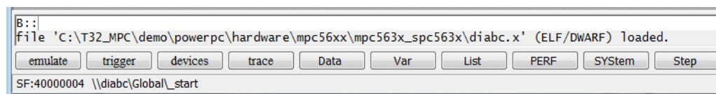
If the boot loader/application is compiled with debug symbols they are automatically loaded into TRACE32 PowerView with the flash programming.
