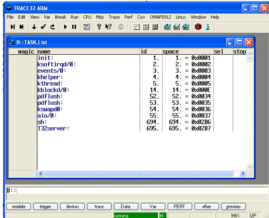
2. Run Mode debugging active (**green M**), selected process (sieve) stopped.
