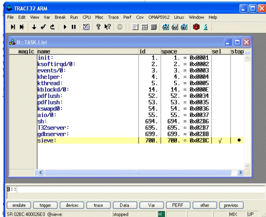
3. Run Mode debugging active (green M), selected process (sieve) running.
