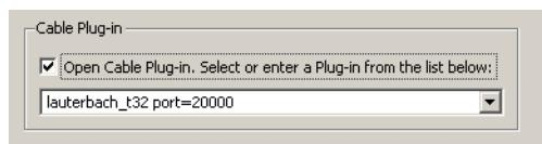
4. Test the plug-in by doing a scan of the target’s scan chain (by right-clicking into the window).
