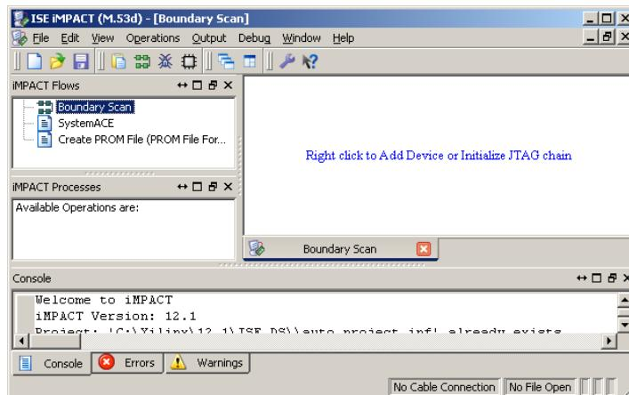
3. Choose **Output** menu -> **Cable Setup** and configure the “Cable Plug-in” box with `lauterbach_t32 port=20000` and click **OK**.
