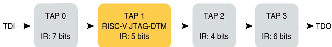
This example shows four TAPs in a JTAG daisy chain. The relevant TAP for RISC-V debugging is the *JTAG Debug Transport Module (JTAG-DTM)* TAP. In order to address this TAP, the following settings are necessary:
