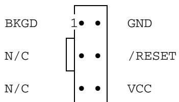
This image shows the top view to the male connector on the target board.
