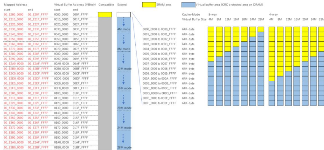
Figure 36.4 The size of SRAM area and Virtual buffer area in the first 1MB area in Extended Mode
